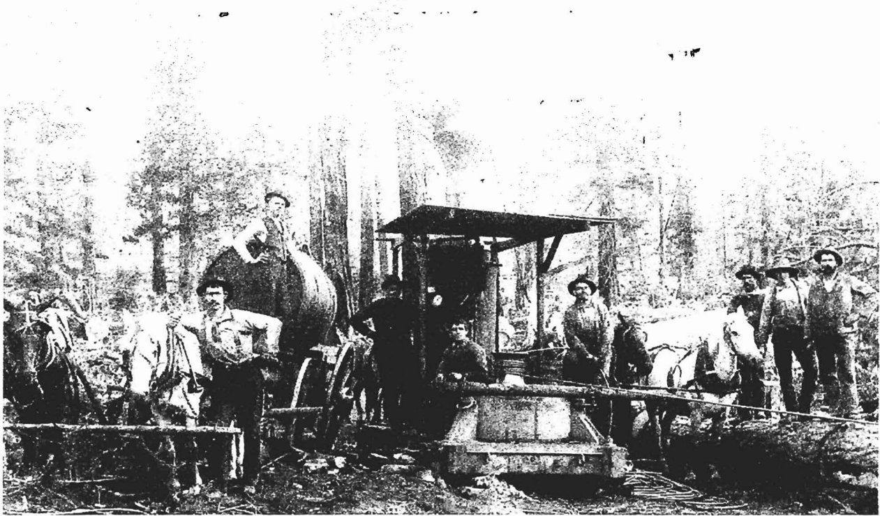
FIGURE 3: Dolbeer donkey engine and Verdi Lumber Company Field Crew ca.1900. [Photo courtesy of Verdi History Preservation Society].
